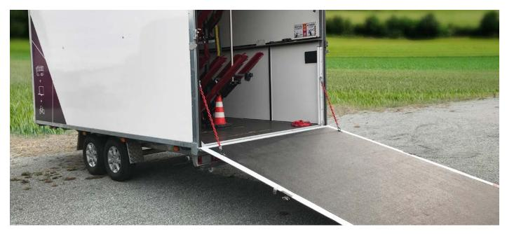
Anti-skid protection even when wet - for safe loading
